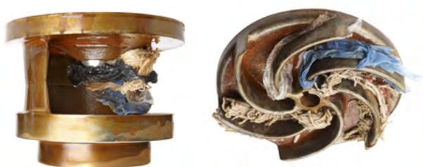
Figure 2: Partial clogging on a single-vane impeller (left) and vortex impeller (right)
