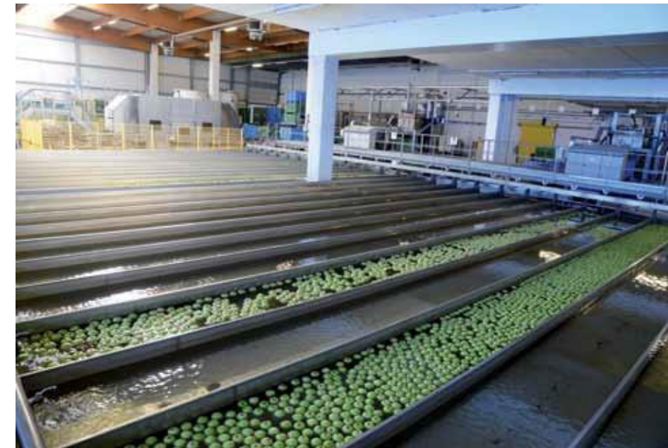
The use of ozone eliminates algae and bacteria without chemical additives or harmful residues
